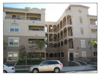
5551 likely applies. Elevated walkway areas designed for humans supported by columns. Note that balconies on left side of photo appear to be within envelope of building, thus not fallable.
